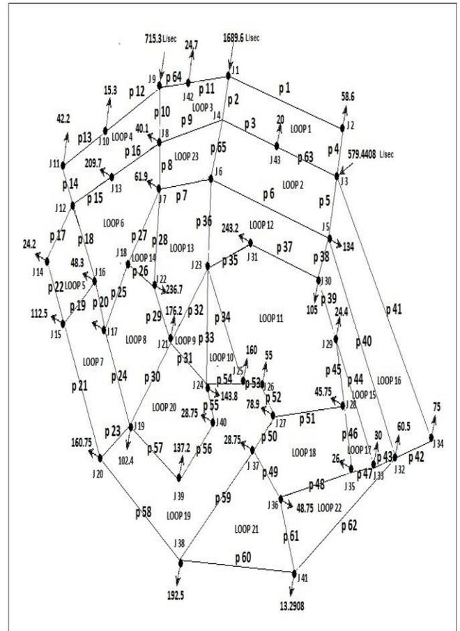
**Figure 1. Configuration of water distribution network and assumed nodal takeoff and direction of flow for water demand for City of Benghazi (year 2014)**
