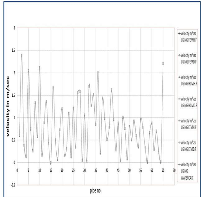
**Figure 3: Comparing the Results of the calculated the velocity of flow in each pipe in (m/sec) using, Finite Element Method (FEMD.F, and FEMH.F), Hardy Cross Method (HCM.D.F, and HCMH.F), and Linear Theory Method (LTMH.F, LTMD.F), and WATERCAD Ready Software**
