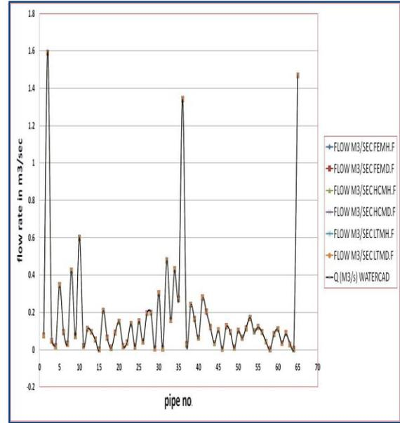
**Figure 2: Comparing the Results of the calculated flow in each pipe in (m<sup>3</sup>/sec) using, Finite Element Method (FEMD.F, and FEMH.F), Hardy Cross Method (HCM.D.F, and HCMH.F), and Linear Theory Method (LTMH.F, LTMD.F), and WATERCAD Ready Software**
