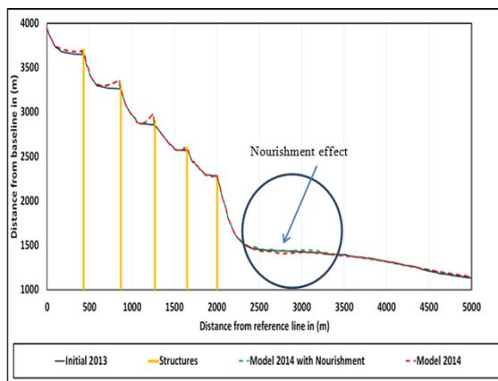
**Figure 10. Model output for using sand nourishment at east Rosetta study area**
