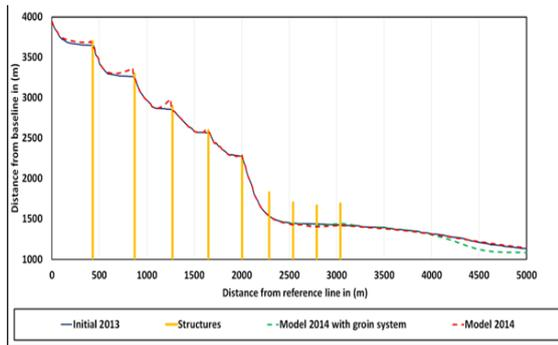
Figure 7. Model output for using groin system at east Rosetta study area
