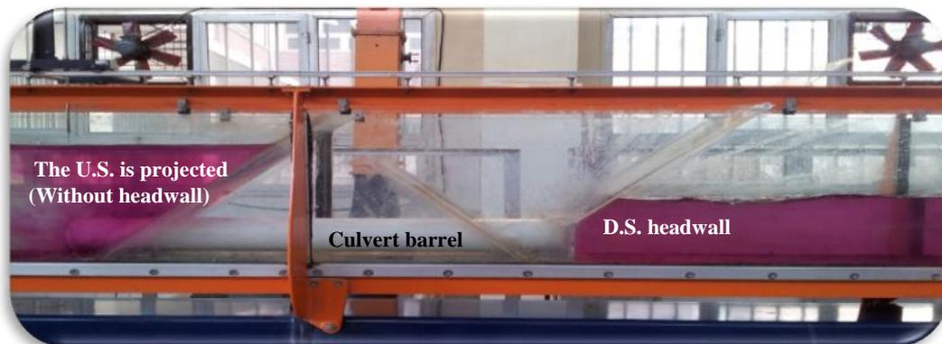
**Photo 2. Testing the effect of D.S. inclined headwall**
