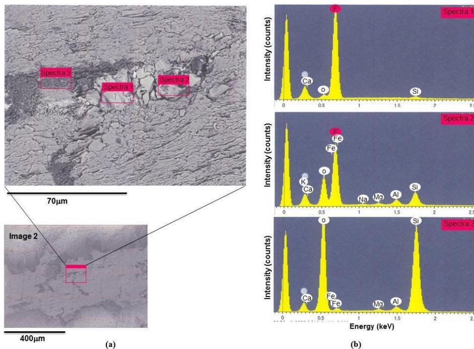
Figure 8. a) SEM image 2 of sample MIZ1-G3 b) Energy dispersive spectroscopy EDS of three different spectra, 70  $\mu\text{m}$ .
