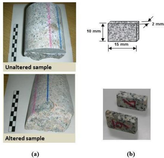
Figure 4. a) Core samples. b) Prepared specimens for the experiment.
