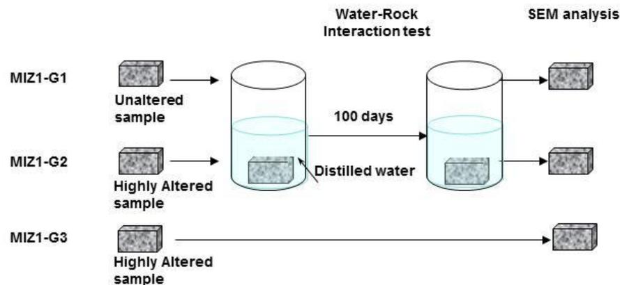
Figure 5. Schematic procedure of the experimental setup.
