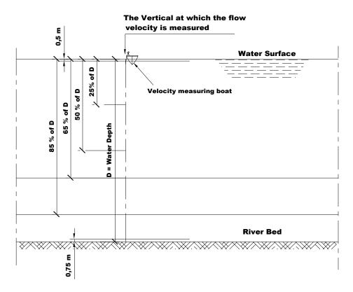
Figure 1. Depths of points along the vertical at which the flow velocity is measured
