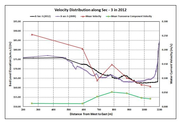
Figure 9. Comparison of Mean Transverse Velocity with Channel Bed Morphological Changes at Sec - 3 in 2012
