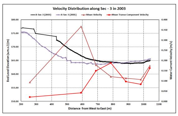
Figure 7. Comparison of Mean Transverse Velocity with Channel Bed Morpholgical Changes at Sec - 3 in 2003.
