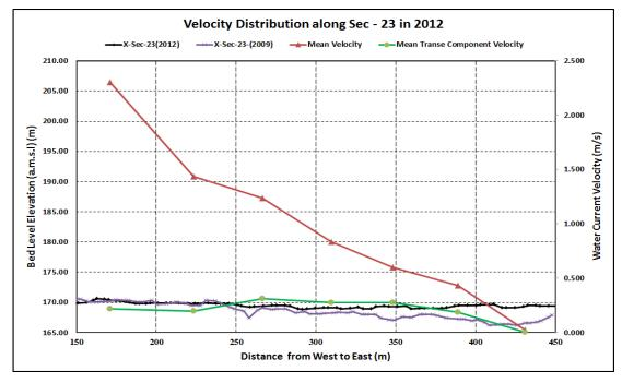
Figure 6. Comparison of Mean Transverse Velocity with Channel Bed Morphological Changes at Sec - 23 in 2012
