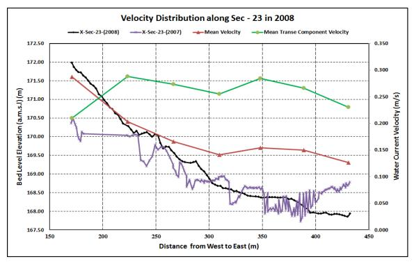
Figure 5. Comparison of Mean Transverse Velocity with Channel Bed Morphological Changes at Sec - 23 in 2008
