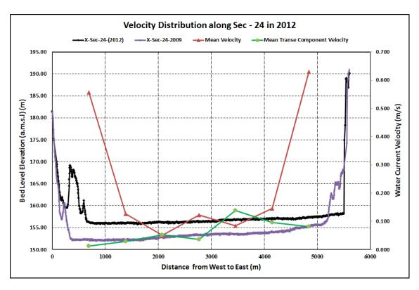
Figure 12. Comparison of Mean Transverse Velocity with Channel Bed Morphological Changes at Sec - 24 in 2012.
