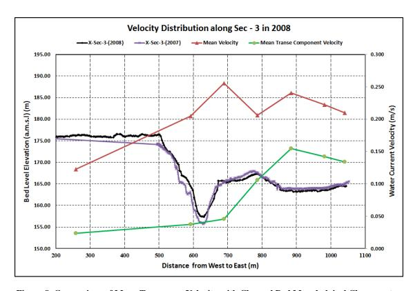
Figure 8. Comparison of Mean Transverse Velocity with Channel Bed Morpholgical Changes at Sec - 3 in 2008.
