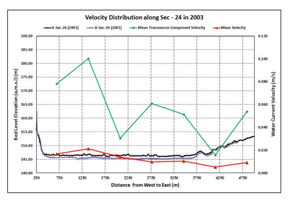
Figure 10. Comparison of Mean Transverse Velocity with Channel Bed Morphological Changes at Sec - 24 in 2003
