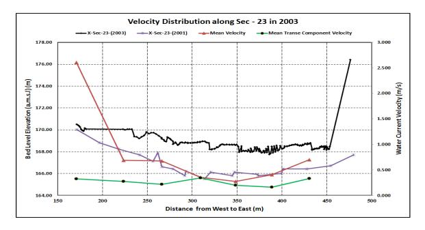
Figure 4. Comparison of Mean Transverse Velocity with Channel Bed Morphological Changes at Sec - 23 in 2003
