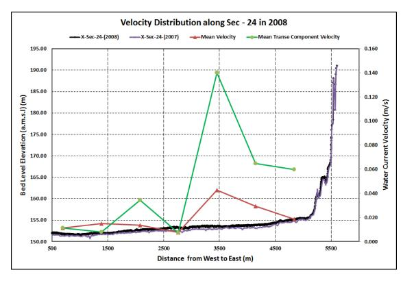
Figure 11. Comparison of Mean Transverse Velocity with Channel Bed Morphological Changes at Sec - 24 in 2008
