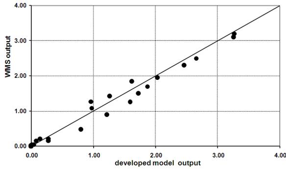
Fig. 16: Comparison between WMS and developed model output (hydrograph)
