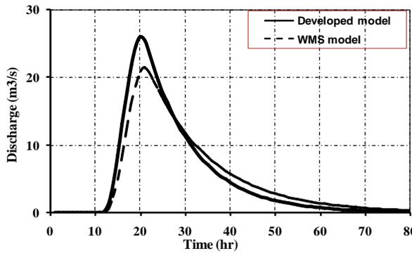
Fig. 25: Comparison between WMS and developed model using Clark equation (storm1)
