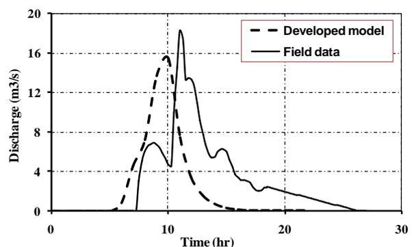
Fig. 30: Comparison between developed model and field data using Nash equation (storm2)
