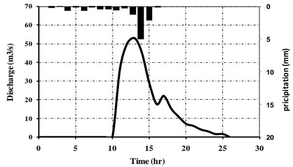
Fig. 20: Observed runoff hydrograph of wadi sudr corresponding to rain fall hyetograph (storm1), (El-Sayed, 2006).
