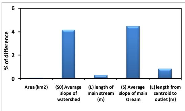
Fig. 24: Percentage of difference between delineation outputs of WMS and developed model (Wadi Sudr)
