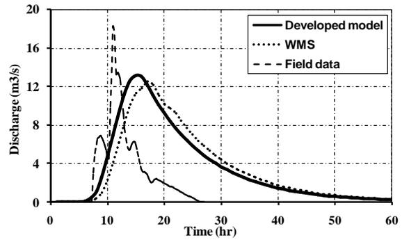
Fig. 32: Comparison between developed model and field data using Clark equation (storm2)
