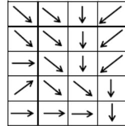
Fig. 3: Flow direction arrows created from the flow direction grid.
