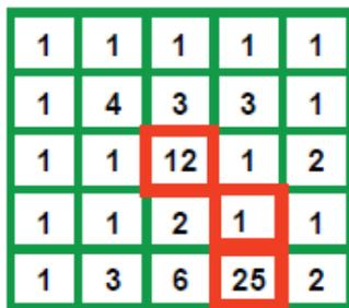
Fig. 4: flow accumulation grid values.
