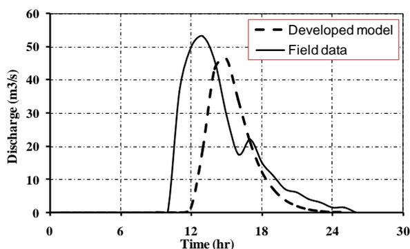
Fig. 29: Comparison between developed model and field data using Nash equation (storm1)
