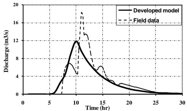
Fig. 34: Comparison between developed model and field data using GIUH equation (storm2)
