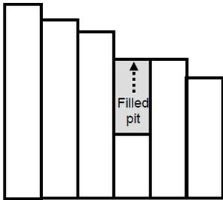
Fig. 1: Cross section of DEM surface.
