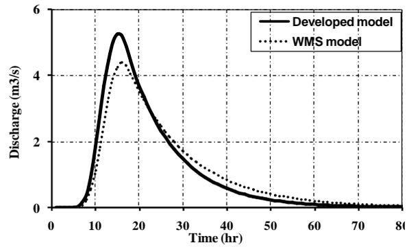
Fig. 26: Comparison between WMS and developed model using Clark equation (storm2)
