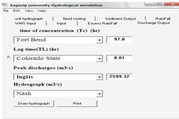
Fig. 8: Lag time, concentration time and runoff hydrograph methods window
