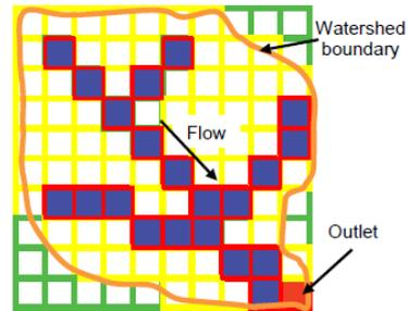
Fig. 5: A grid representation of a watershed boundary, stream network and outlet.
