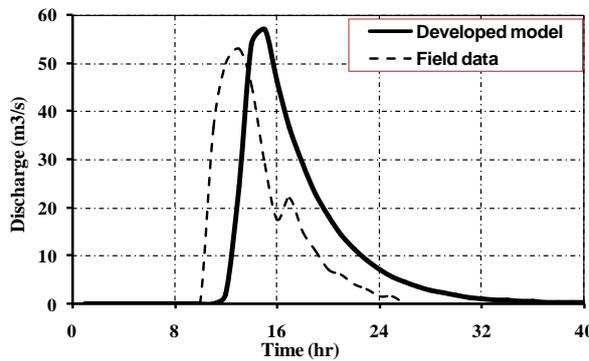
Fig. 33: Comparison between developed model and field data using GIUH equation (storm1)
