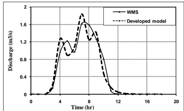
Fig. 15: Comparison between WMS and developed model hydrographs case (2)
