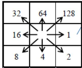
Fig. 2: Direction codes (integer numbers) assigned to cells in flow direction grids.
