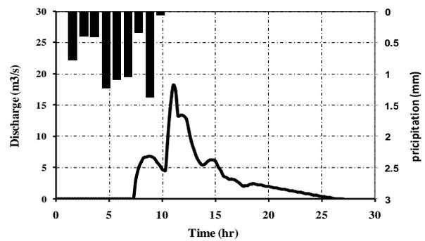
Fig. 21: Observed runoff hydrograph of wadi Sudr corresponding to rain fall hyetograph (storm2), (El-Sayed, 2006).
