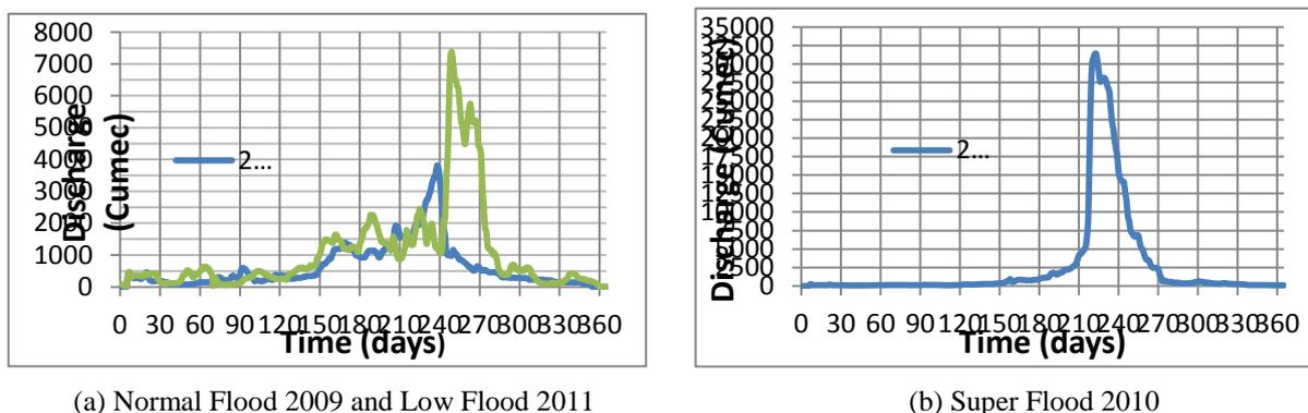
Figure 3. Observed annual flow for year 2009, 2010 and 2011 at downstream Sukkur barrage
