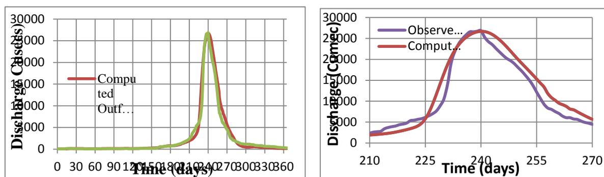
Figure 5. Computed and observed outflow hydrograph at upstream of Kotri barrage in year 2010
