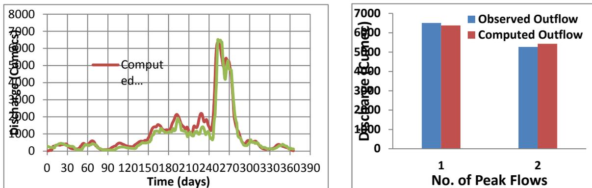
Figure 6. Computed and observed outflow hydrograph and two major peaks for the year 2011
