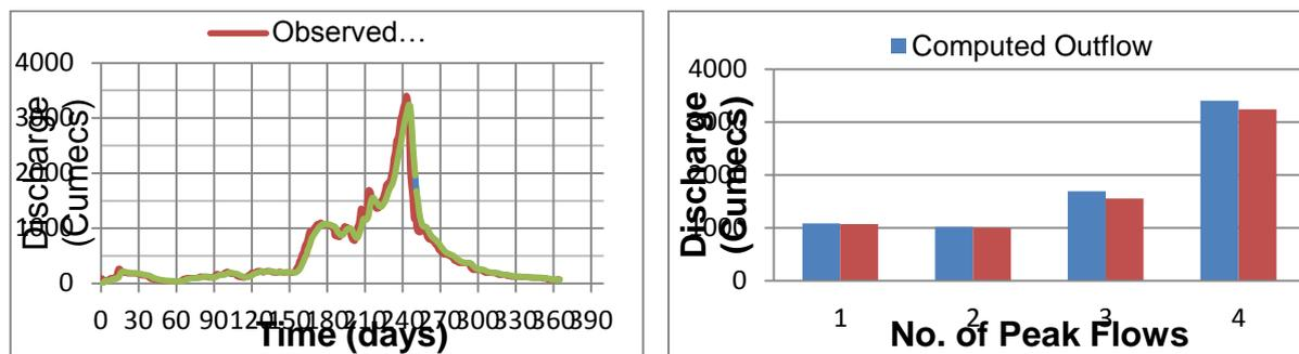
Figure 4. Computed and observed hydrographs at upstream of Kotri barrage along with peaks in 2009
