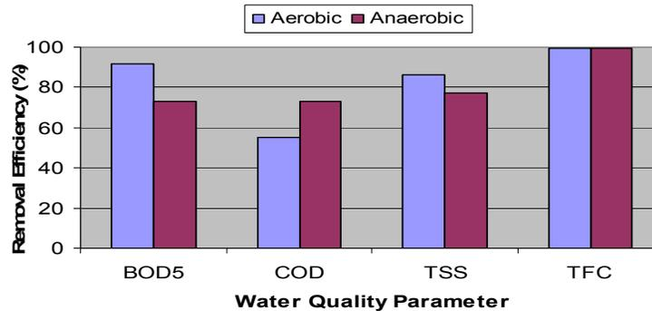
Figure 4 Average Removal Efficiency of Aerobic and Anaerobic Wastewater Treatment Plants
