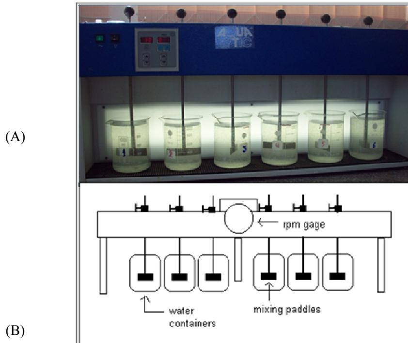
**Fig. 1 The laboratory floc tester: (A) photo, (B) schematic diagram**
