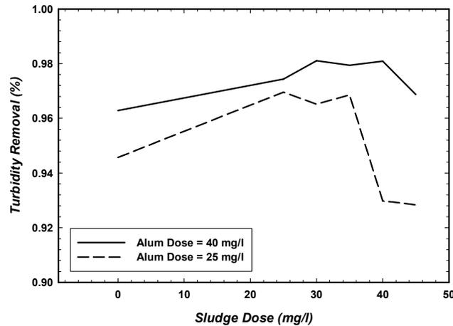
Fig. 3 Turbidity removals at different sludge dosing with two different alum dosages
