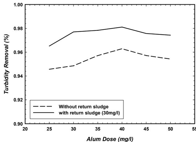
Fig. 2 Turbidity removals with and without sludge dosing at different alum dosages
