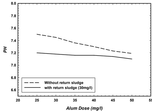
Fig. 4 pH values with and without sludge dosing at different alum dosages
