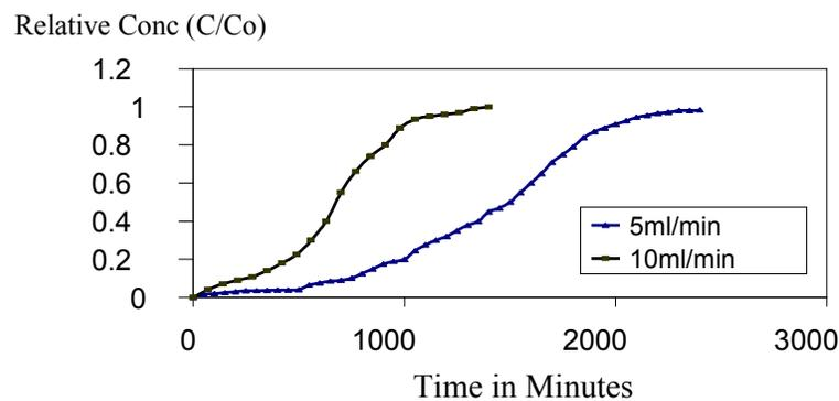
Figure 6. Break through profile for adsorption of Fluoride by column filled with Rice Husk
