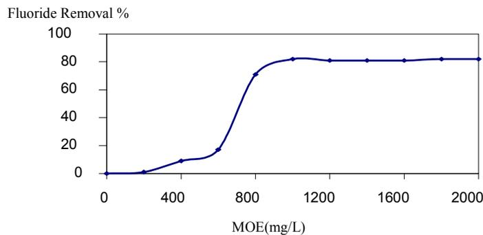
Figure 7. Effect of coagulant dose on Fluoride removal by *Moringa oleifera*.
