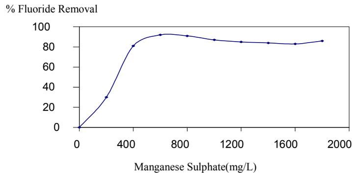
Figure.12 Effect of Manganese sulphate dose on fluoride removal at optimum pH
