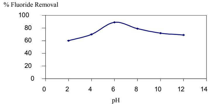
Figure 11. Effect of pH on coagulative removal of fluoride by Manganese sulphate
