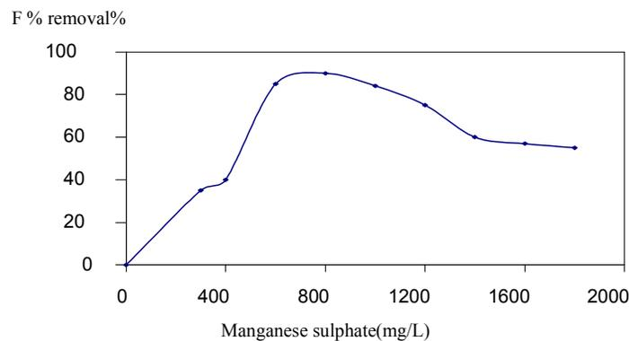
Figure.10 Effect of coagulant dose on fluoride removal by Manganese sulphate
