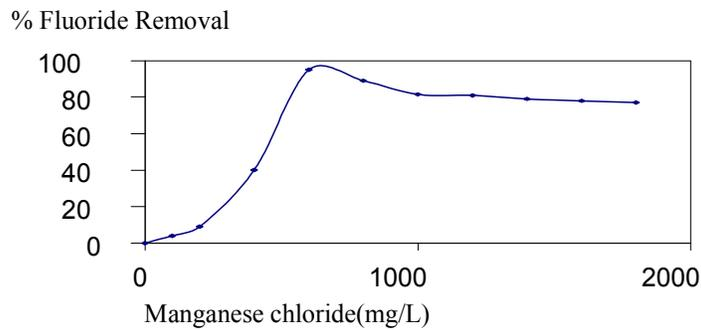
Figure.15: Effect of Manganese chloride dose on fluoride removal at optimum pH
