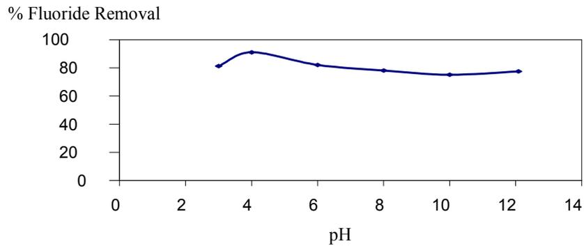
Figure.14 Effect of pH on coagulative removal of fluoride by Manganese chloride
