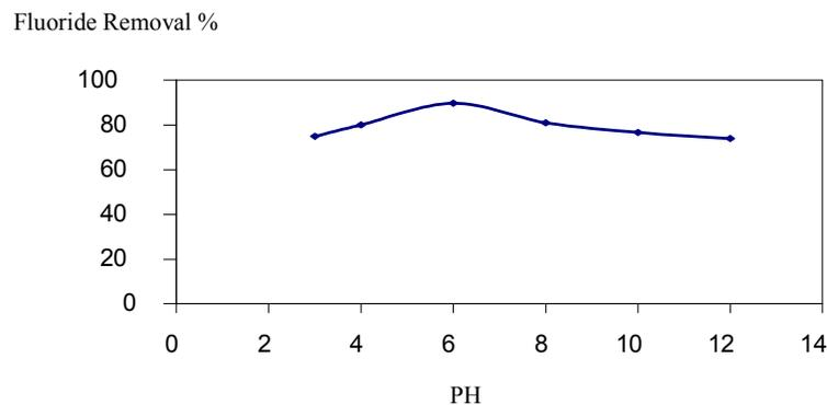
Figure 8. Effect of pH on coagulative removal of Fluoride by *Moringa oleifera*.
