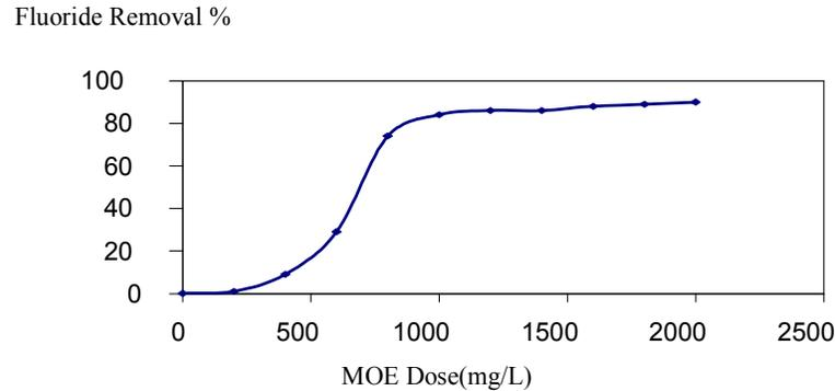
Figure.9 Removal of fluoride by *Moringa oleifera* Extract at optimum pH
