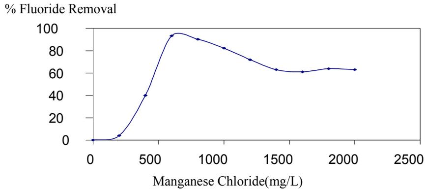
Figure.13 Effect of coagulant dose on Fluoride removal by Manganese chloride
