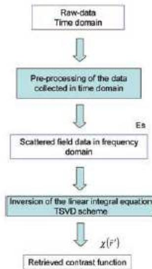
Fig. 2 The processing chain from the time-domain raw data to the contrast function
