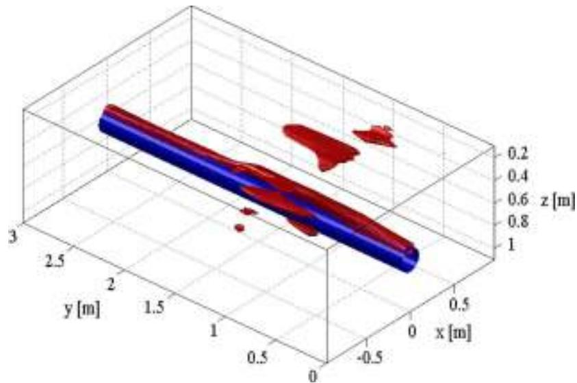
Fig. 3 (Red) Three-dimensional image of the (blue) pipe as a result of the superposition of all the 2-D reconstructions (scans from S1 to S7).
