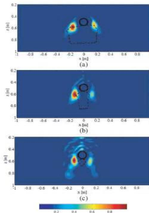
Fig. 5 Normalized modulus of the reconstructed contrast achieved through the distorted wave tomographic approach in the three cases of a (a) large; (b) medium, and (c) small leak.
