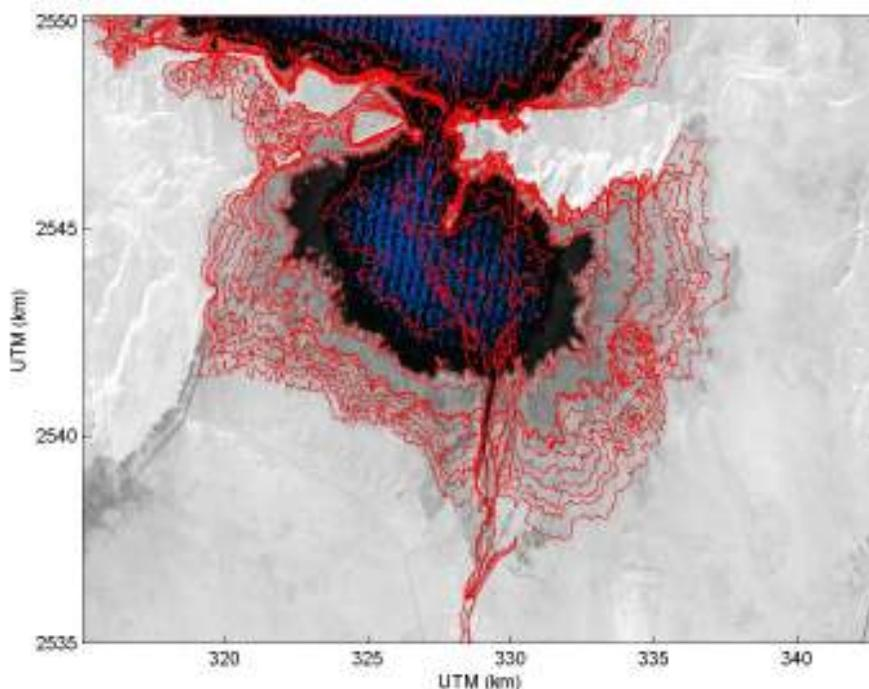
**Fig. 9 Toshka Lake 1 bathymetry 5-m contours intervals**
